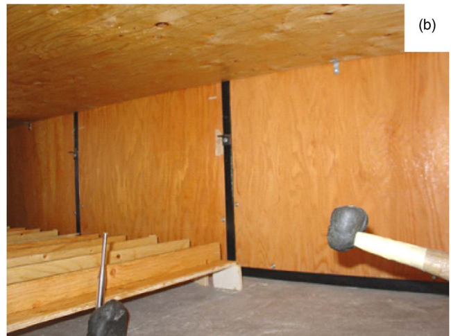
FIG. 2. (Color online) Photographs of the 1/8-scale model without ceiling baffles or reflectors: (a) showing the seats and rear partition; (b) showing the model speech source and microphone.
